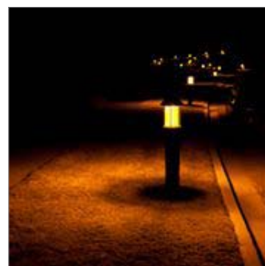
Figure 4: The Mount John Village subdivision, which is lit by bollards that comply with the requirements of the observatory (Fraser Gunn).
