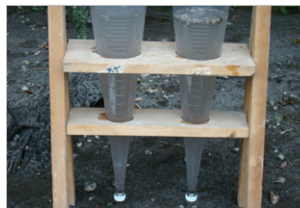
Use of plastic graduated cones to evaluate loads of sedimentable material
