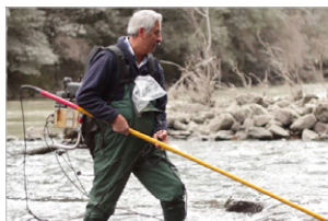
Use of electric shock fishing machine to analyse fish communities
