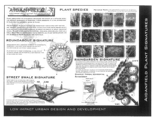
Figure 5. Plant signature for roundabout, street swale and rain garden in Aidanfield subdivision. Design: F Baggaley, 2006
