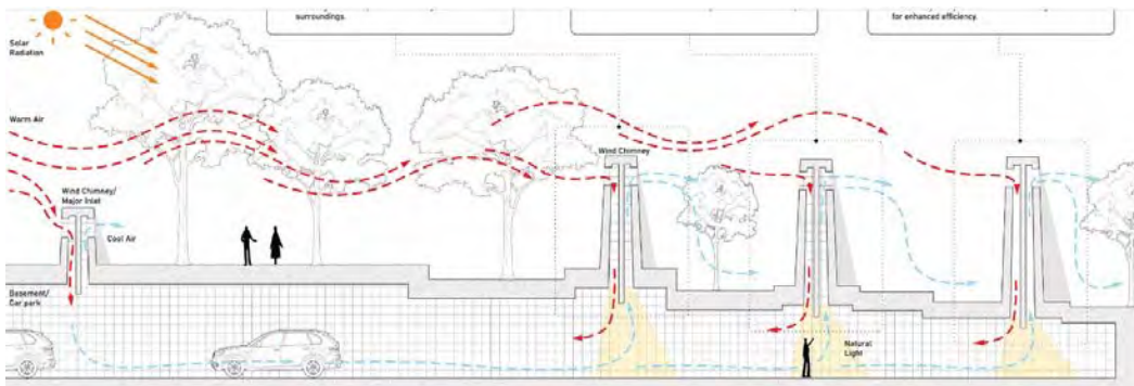
Figure 6. Student design showing air flow moving up and down proposed chimney structures (image from Designing for Heat intensive subject , 2023).
