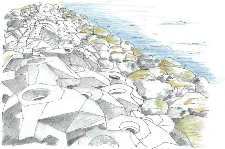
Figure 8. Modified Xbloc revetment section against the new pathway (sketch by author).
