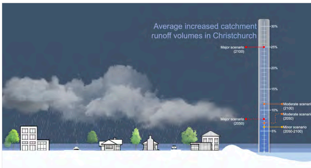
Figure 2. Substantial flooding is projected to occur in many low-lying coastal cities of Aotearoa New Zealand. In Christchurch by 2050, runoff volumes corresponding to different rainfall events were projected to increase by between 6 per cent under the minor scenario (+1 degree Celsius by 2100) and 8 per cent under the major scenario (+4 degrees Celsius by 2100). While the impact associated with the minor scenario would remain steady after the middle of this century, increases in runoff volumes would reach about 10 per cent under the moderate scenario (+2 degrees Celsius by 2100) and 25 per cent under the major scenario by the end of this century (image by Suphicha Muangsri, 2023).
