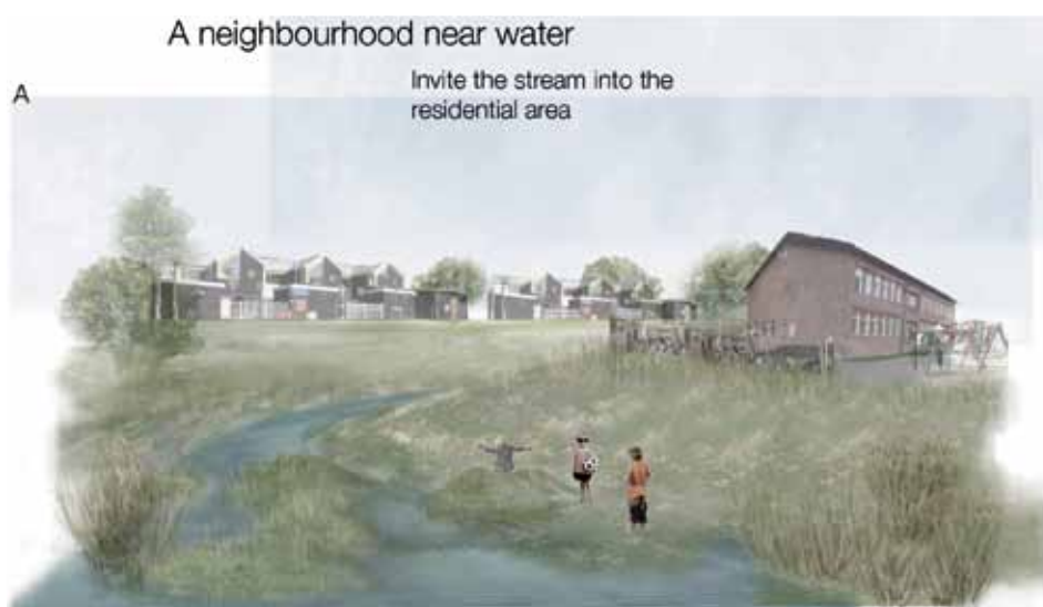
Figure 3b: The proposal by Elise Eriksson is based on her previous studies and visualisation of a coastal landscape with sections (see above). Houses are placed on higher ridges in the new landscape, while sea water can find its way in between. The landscape can still be used and the confrontation with the sea is minimised. (Image: Elise Eriksson.)
