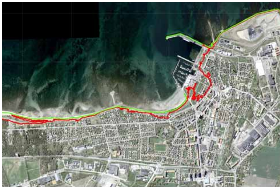
Figure 1: The red line on the map represents the idea about the future coastline in around 100 years, when the sea is at its highest. The line is static (in the same way as the actual coastline on the map) and does not communicate the dynamics of the coastal landscape. (Map: DHI for Höganäs municipality.)
