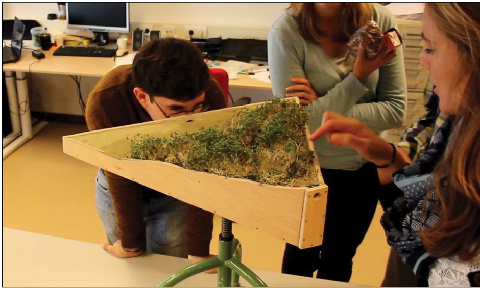
Figure 4: Interaction with the physical-scale model, in collaboration with Jolanda de Jong, including a water circulation, a wooden base, sand topography, cardboard paths and cress vegetation. (Image: Author's own.)
