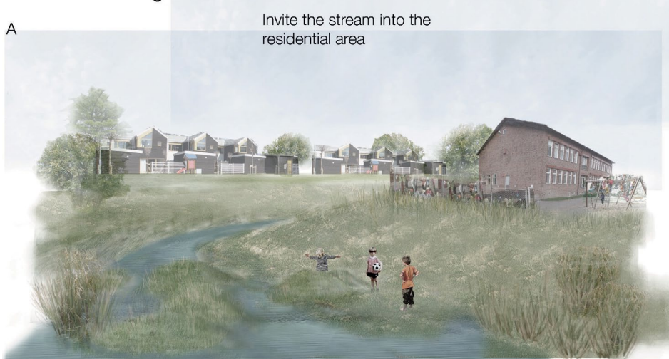
Figure 3b: The proposal by Elise Eriksson is based on her previous studies and visualisation of a coastal landscape with sections (see above). Houses are placed on higher ridges in the new landscape, while sea water can find its way in between. The landscape can still be used and the confrontation with the sea is minimised. (Image: Elise Eriksson.)
