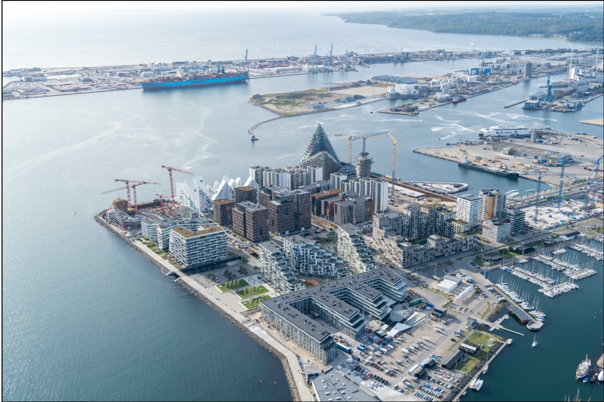
Figure 1: Photos of current waterfront residential development models in the coastal city of Aarhus in Denmark. The residential and commercial development on Aarhus Docklands (Aarhus Ø) started in 2007 on a former container terminal that was reclaimed land. It is 100,000 km 2 with plans to house over 10,000 residents. The Docklands is elevated 2.5m above the previous normal water level based on a future increase in sea level of 0.5m with stone reefs as coastal protection to dampen the waves. However, the Docklands is considered a storm surge risk area, and it seems to be underestimated to deal with future predictions of SLR and storm surges by the end of the century (Aarhus Kommune, n.d.; Klimatilpasning, 2015). Aerial photo of Aarhus Docklands by Jesper Larsen and JFP.dk.
